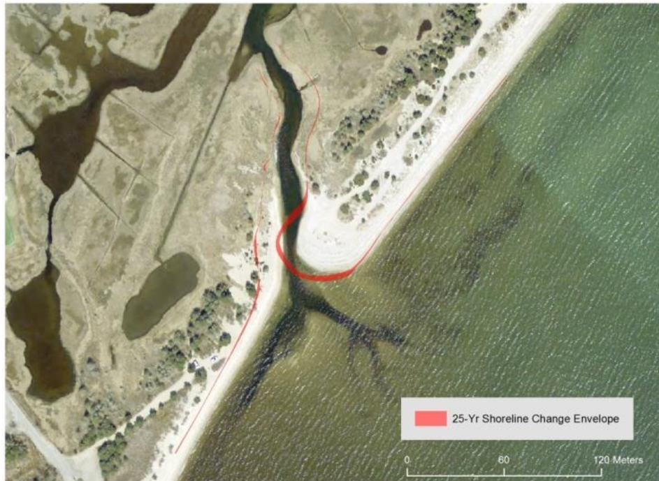
Figure 3-3: Envelope of potential shoreline positions at the 25-year time horizon based on the range of calculated shoreline change rates.
