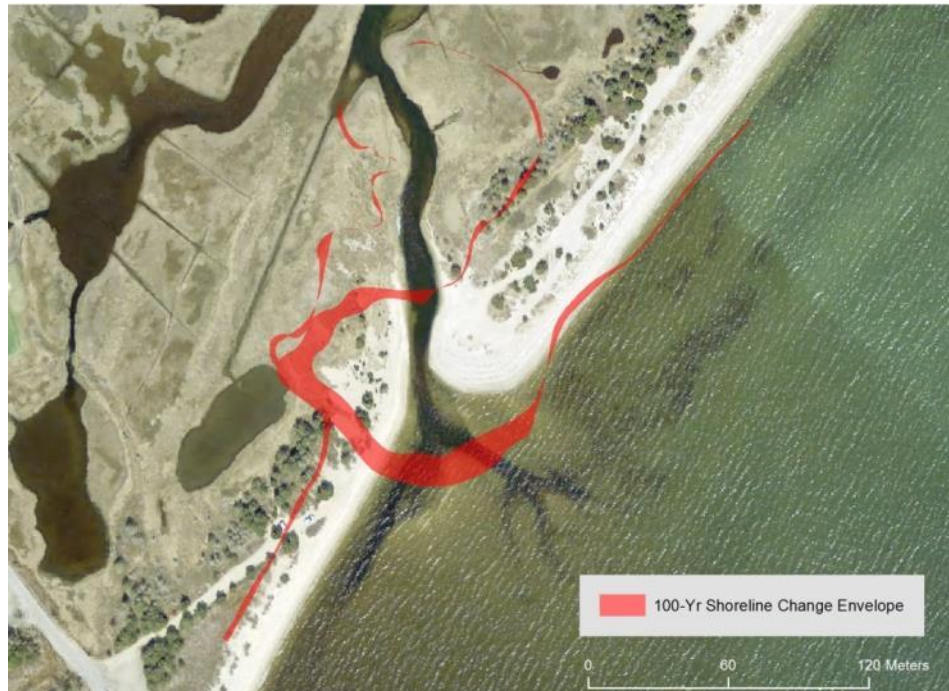
Figure 3-5: Envelope of potential shoreline positions at the 100-year time horizon based on the range of calculated shoreline change rates.
