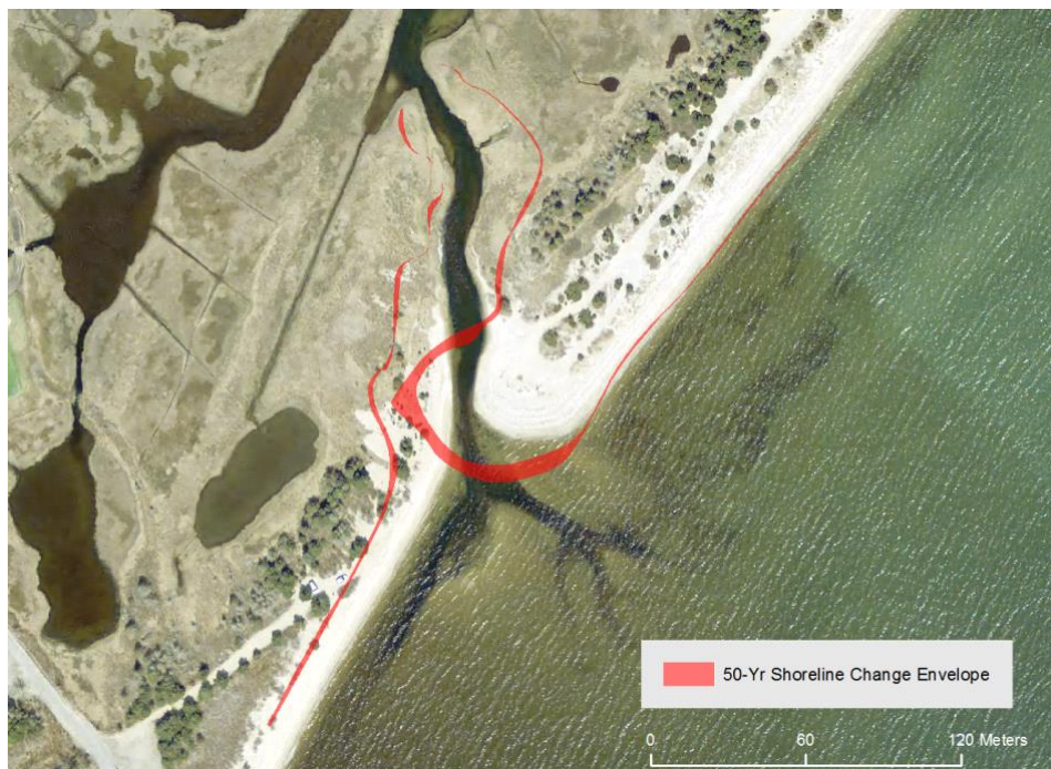
Figure 3-4: Envelope of potential shoreline positions at the 50-year time horizon based on the range of calculated shoreline change rates.
