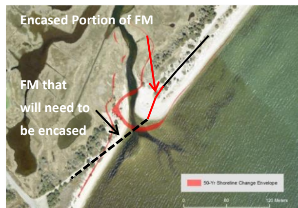
Figure 3-28: Example showing the predicted 50 year shoreline migration and the portion of the sewer line that would need to be encased
