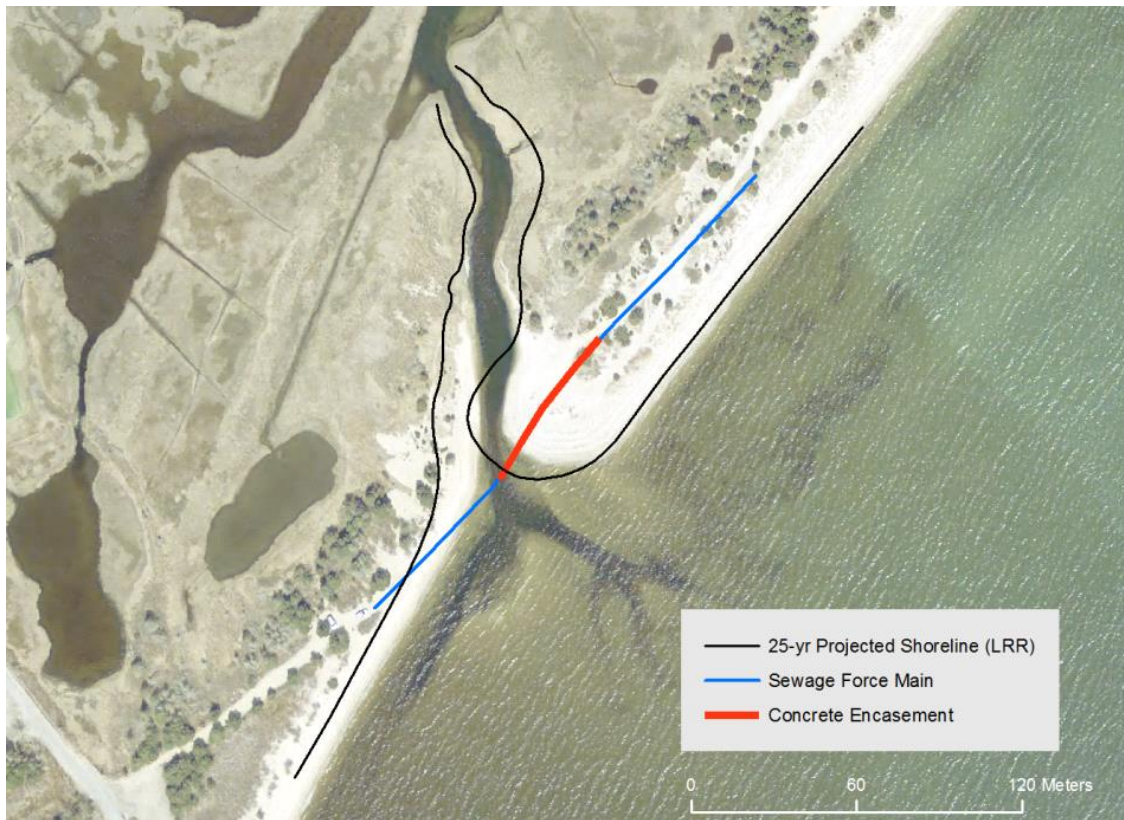
Figure 3-2: Projected shoreline configuration at the 25-year time horizon using LRR rates of change. The position of the sewer force main (including extent of armoring) is based on plans (data provided BBNEP).
