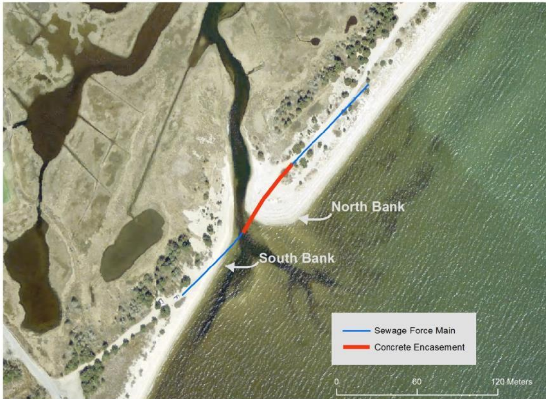
Figure 2-4: Diagram of the sewer line along the Eel Pond Inlet. Data showing locations of the force main and encasement was provided by BBNEP.
