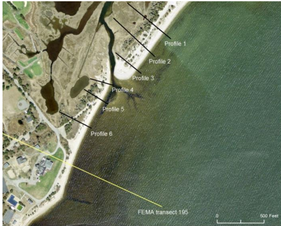
Figure 3-7: Location of cross-shore profiles on either side of the inlet and FEMA transect used to estimate SWEL.
